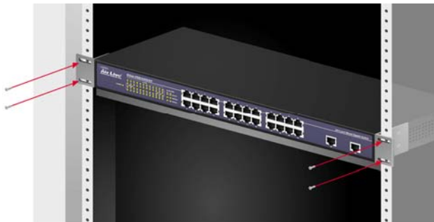
Figure 3. Mount the Switch in the rack
