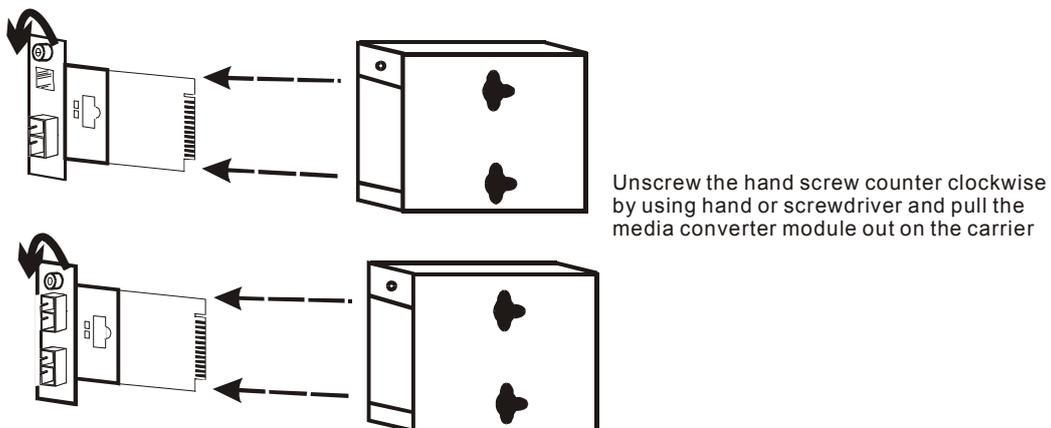
**Step 3:** Carefully slide in the module and fasten the hand screw clockwise by using hand or screwdriver until it is fully and firmly fitted into the slot of the chassis.
