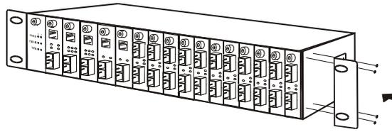
**Step 2:** Carefully position the chassis into the rack. Align the brackets to the side holes on the rack and use rack screws to secure the chassis with the rack.
