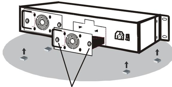
You can slide in and out the power supply from the bay, fasten or loose the hand screw clockwise or counter clockwise by using hand or screwdriver.
